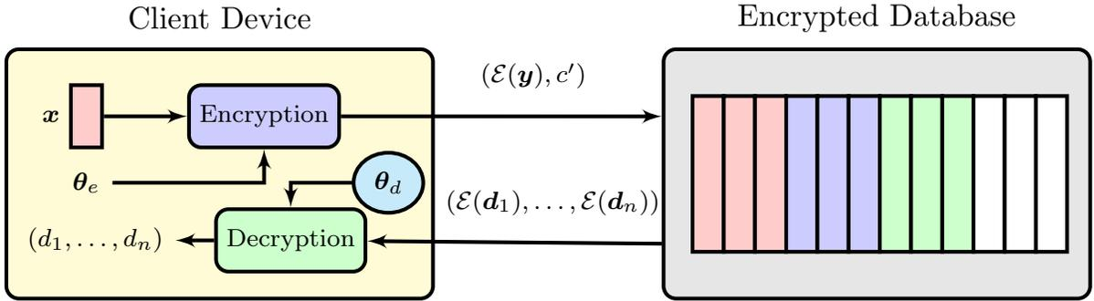
(b) **Authentication:** During this phase, a user seeks to get authenticated, encrypts the probe feature vector with the public key  $\theta_e$  and transmits to the database along with the claimed identity. The database computes the dissimilarity score over encrypted features and transmits the matching score to the client, where it is decrypted with the private key  $\theta_d$ .
