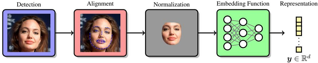
Figure 1: A typical **face representation pipeline** comprises of face detection, alignment, normalization and feature extraction. The embedding function maps a high-dimensional normalized face image to a  $d$ -dimensional vector representation.
