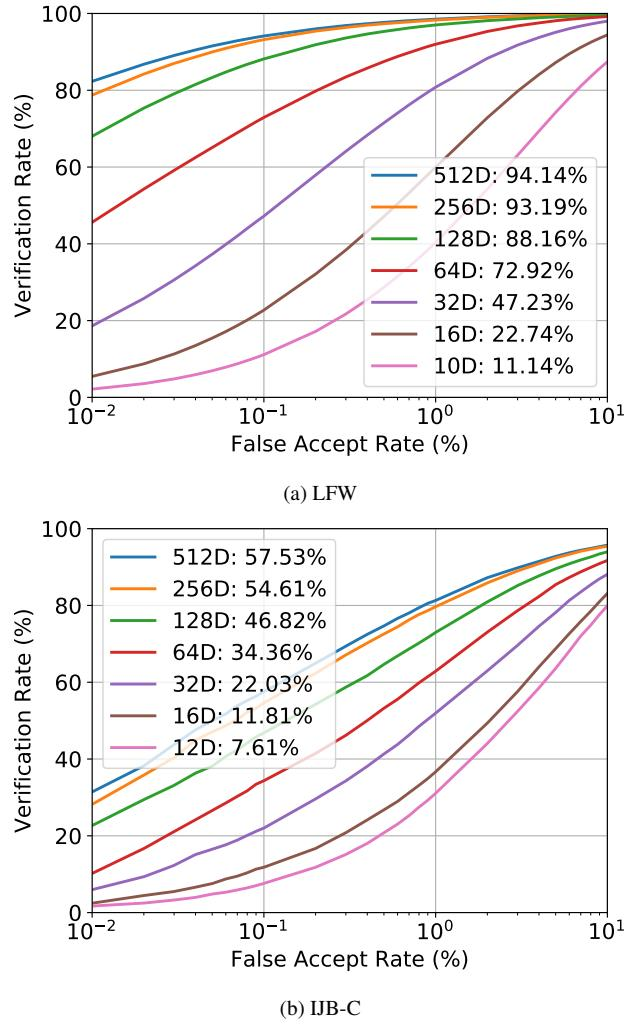
Figure 1: ROC curve on LFW and IJB-C datasets for the Inception ResNet V1 [5] model trained with different embedding dimensionality on the CASIA-WebFace [8] dataset.
