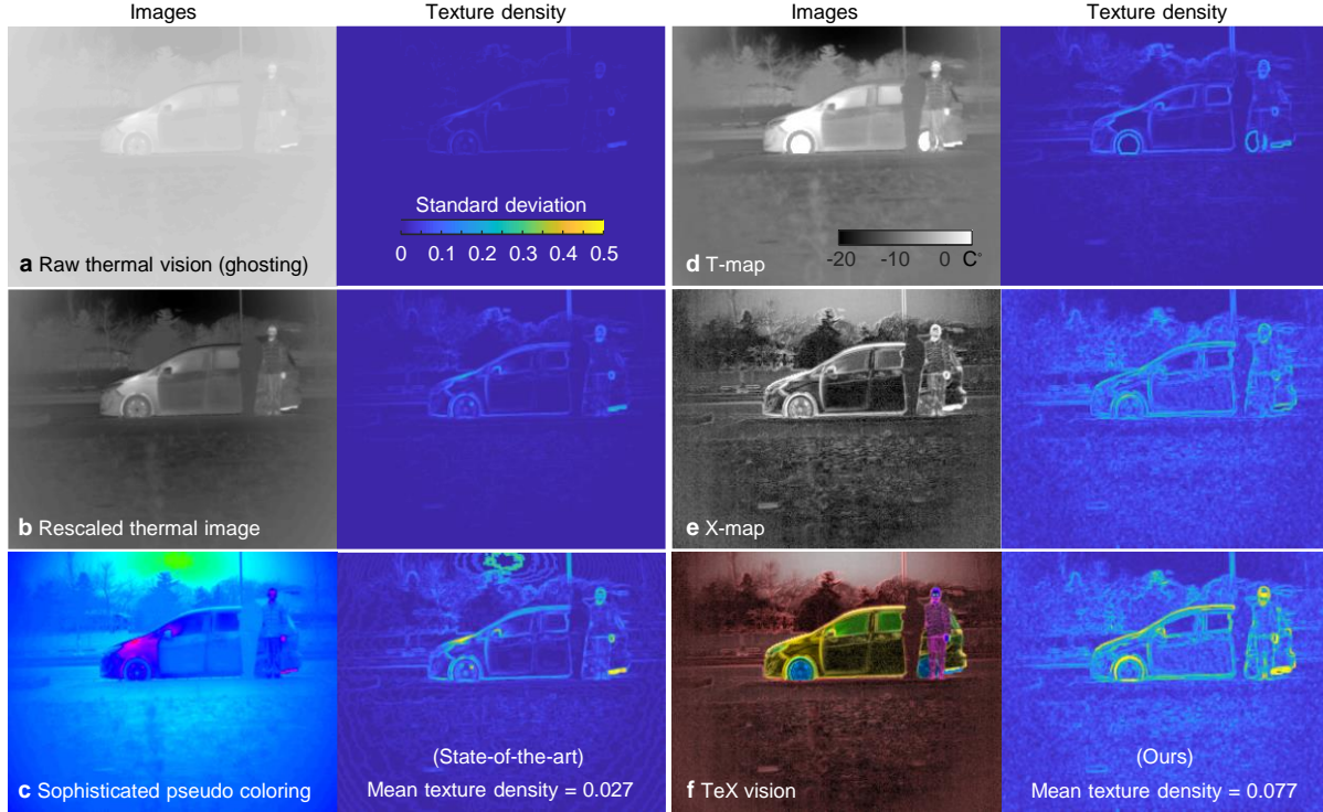
FIG. S13. Experimental HADAR TeX vision at a winter night (Dec. 2020, Indiana, USA) beats conventional thermal vision in textures. a, Raw thermal vision of a winter night scene taken by FLIR camera A325sc. b, Rescaled thermal image to improve the visual contrast. c, Empirical pseudo coloring (HSV, Matlab) adopted by modern thermal cameras to improve the visual contrast. d-f, HADAR T-map, X-map, and TeX vision taken by our HADAR prototype-1. The texture density value at each pixel is the standard deviation of the corresponding 3 \times 3 neighboring pixel array. Our TeX vision gives a texture density of 0.077 on average over the whole image, better than the state-of-the-art pseudo coloring approach which has a texture density of 0.027 on average. Note that more textures means more details in images but means higher values in texture density, so the brighter the texture density figure, the better. Errors remaining in texture (e) are due to mismatch of the emissivity profiles in the real scene with the material library, as well as multi-object scattering contributions, and consequently they are obvious around boundaries. This can be overcome in the future by on-site calibrations of the material library and more advanced decomposition algorithms.
